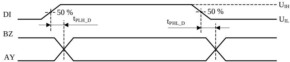
Figure 3 – Timing diagram for measuring t_{PLH\_D} and t_{PHL\_D}
